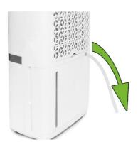
When using the drainage hose, make sure that there is a continuous slope of the hose to ensure proper emptying. The water hose can be directed to a floor drain or other suitable drain. In any case, the drain must be lower than the condensate connection of the unit.
