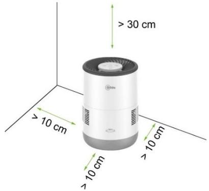
2. To ensure optimal performance of the device, please ensure that the air inlets and outlets are not covered.
